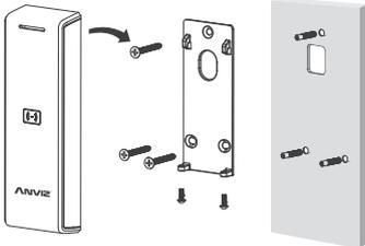
1. Drill outlet hole on the wall for device wiring and 3 screw holes on the wall according to the mounting bracket.
