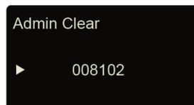
**Note:** in admin clear interface, you can press [OK] key to input admin ID and delete it manually. Press [OK] key again and confirm to delete manager 8102. Then exit to manager clear interface.
