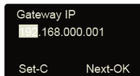
Press [**<**] or [**>**] key or number key to input gateway IP. Press [**OK**] key to shift between the 4 segments. After set is completed, press [**C**] key to enter gateway IP save interface.
