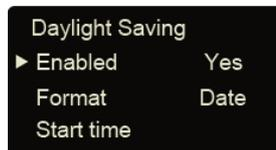
When you enable 'Daylight Saving' function you need select week or date format first. Then you need set the time point for 'Daylight Saving' start time and end time. And press [C] key enter save interface.
