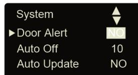
Press [<] or [>] key or number key to input door alert value. Press [OK] key to confirm. Then press [C] to save the setting.
