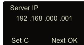
Press [<] or [>] key or number key to input server IP. After set is completed, press [C] key to enter save interface.
