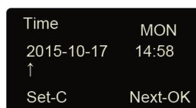
You can press the [OK] key to move the cursor to shift the year, month, day. And use number and [<] or [>] key adjust the time. After setting completed, press [C] key and enter system time save interface.
