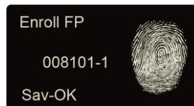
Press [**OK**] to save fingerprint. Press [**C**] back to user registration interface. The 2nd finger registration as the same steps as above.
