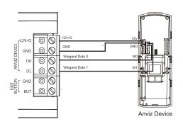
Notice: Please install the power cord and the cable in accordance with the marks, Incorrect way of installation would damage to the equipment.
