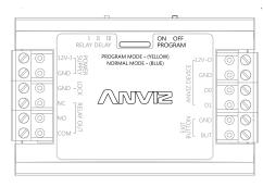
Switch in 'PROGRAM MODE' on the SC011: Move slide switch to left(ON).
